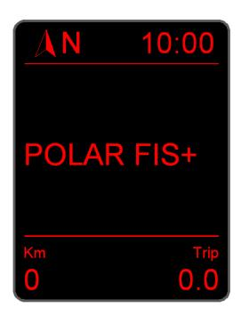
Inside this screen, using the UP and DOWN buttons, you can modify each letter of the text, modify the first character, and after that make a short press of OK button, this will allow you to modify the next character, and each OK short press will change the character to edit. Once you have finished editing the text, press and holding OK button until a screen prompts asking you to change the name.
