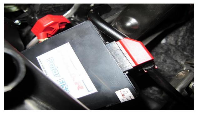
As you can see in the photography, PolarFIS has 2 connectors, you must connect the connector which you just extract from the Gateway in one of the free PolarFIS connectors (either of them is valid), next, you must connect one of the ends of the cable to the connector that is free in your PolarFIS and the other end must be connected to the Gateway.
