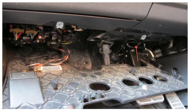
Once the inferior cover is removed, we will have to locate the connection of the Gateway for "bypassing it" with PolarFIS. (see further on).
