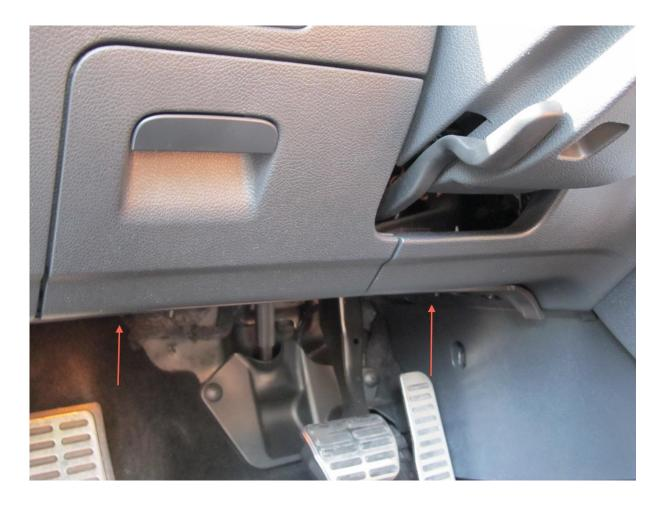
This cover has two Torx screws, and it falls throwing towards underneath.
