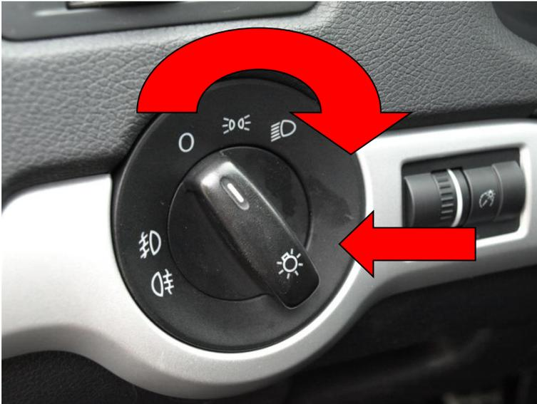
In order to extract the control, push the handle towards inside, maintain the pressure and turn the control towards the right side until this approximately indicates the position of dipped headlights. Next throw towards outside and the control will be completely out.
