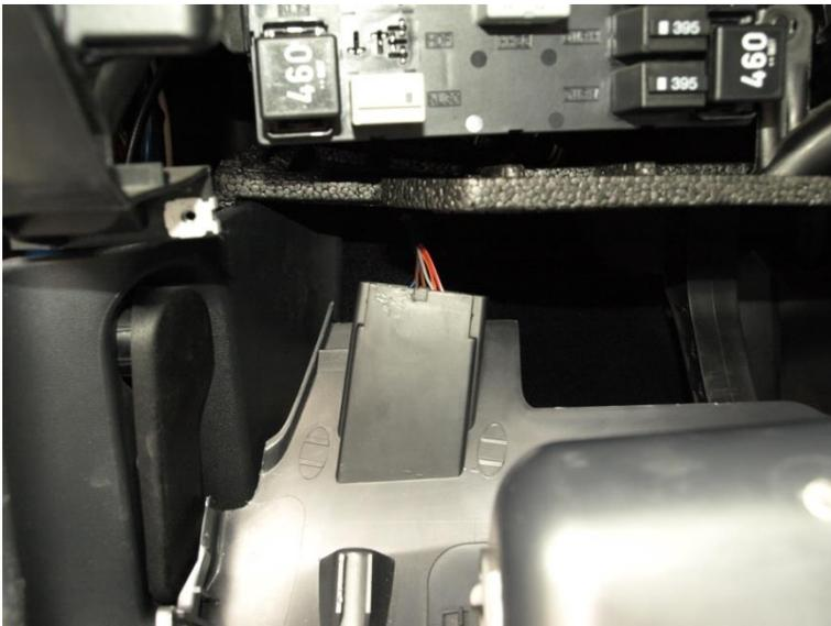
In order to loosen this connector, you must press, with a screwdriver, in the points indicated in the following image, while the connector is pushed towards inside.
